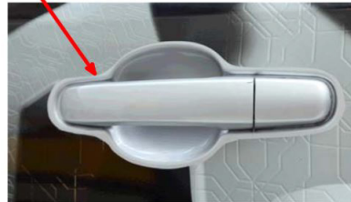
Tenting over door handle Lifting in deep contours
